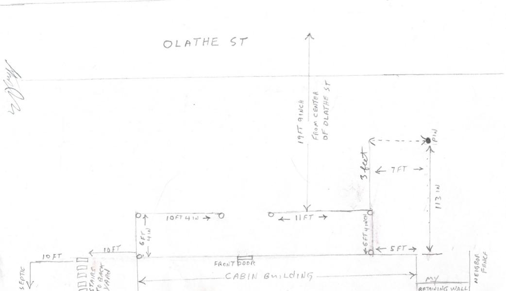
PROPOSED SPLITRAIL FENCE AT 10880 OLATHE ST.
